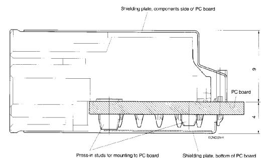
Shielding plates can at a later time be attached to the female connector already pressed in. The fully equipped female connector with the grounding/shielding plates has 6 rows on the terminal side. The grounding pins are in a 5.0-mm grid.
