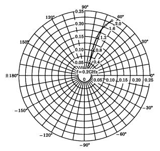
$\begin{array}{l} \text{S}_{22e} \\ \text{V}_{\text{CE}} = 10\text{V} \\ \text{I}_{\text{C}} = 20\text{mA} \\ \text{Ta} = 25^{\circ}\text{C} \\ \text{(UNIT}: \Omega) \end{array}$
