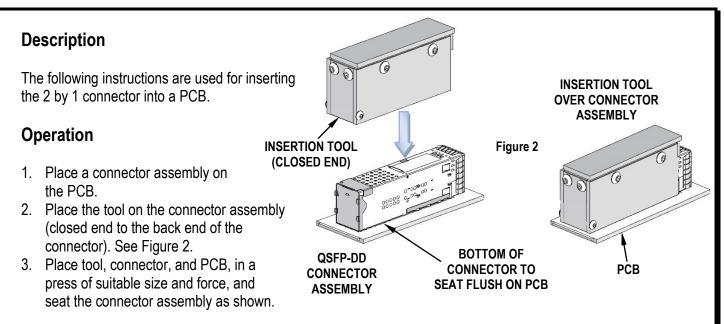
The support plate (furnished by the customer) under the PCB must have clearance for the connector pins as they pass through the PCB.
