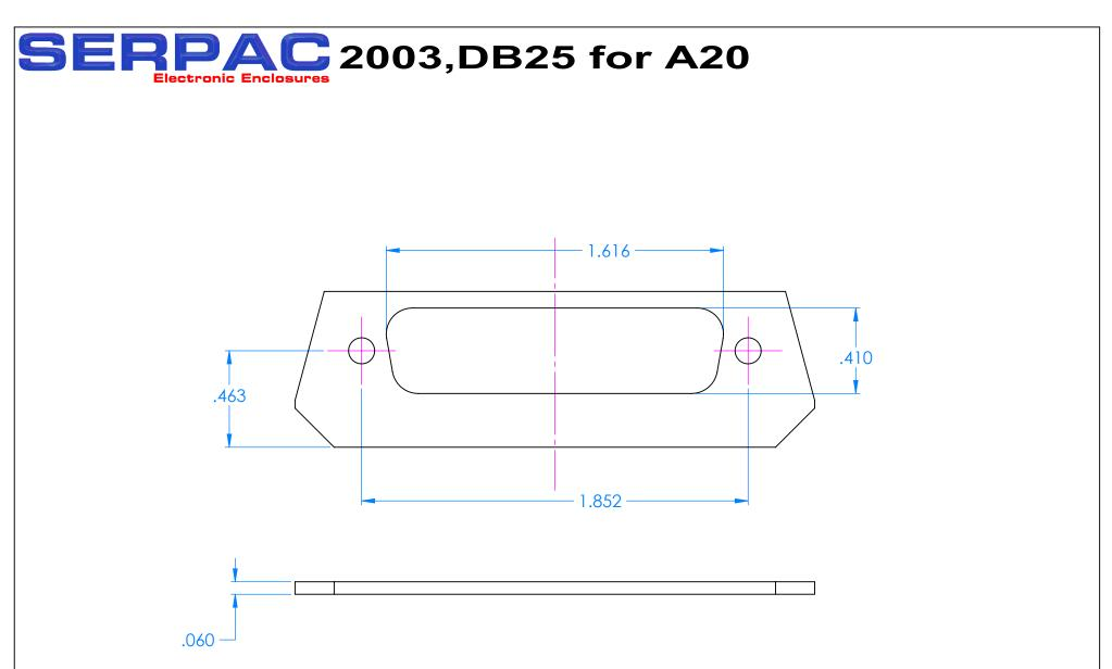
NOTES: Cutout located to accept a D-sub standard surface mount DB25 connector (male or female) using a .065" thick circuit board.
