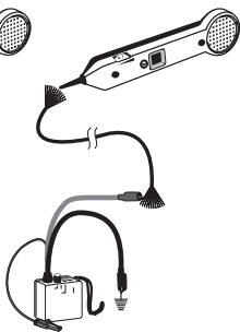
Figure 2b. Cable Tracing
