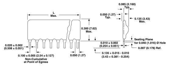
Pin #1 is extreme left-hand terminal on side with marking.
