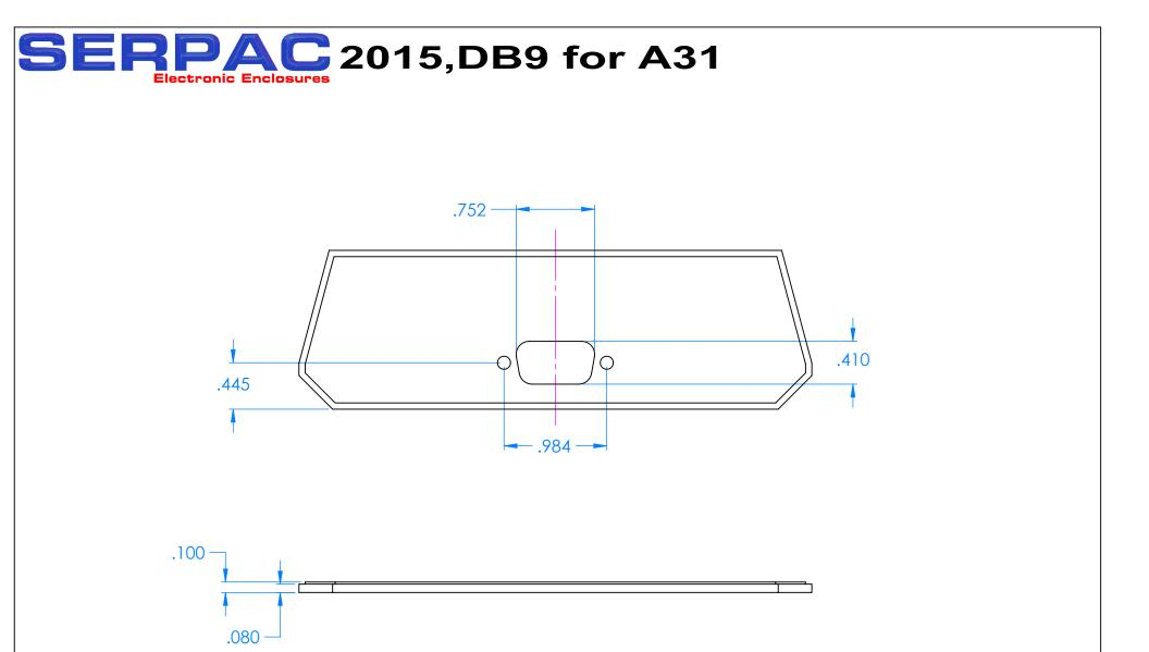
NOTES: Cutout located to accept a D-sub standard surface mount DB9 connector (male or female) using a .065" thick circuit board.
