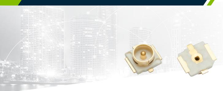
Part of the Taoglas SMD Mount Receptacle, the RECE.20279.001E.01 is a 3-pad type wire-to-board SMD receptacle that is ultra-small, lightweight and low profile, 2.5mm max. With an operational frequency range of DC to 6 GHz the RECE.20279.001E.01 is gold plated to provide superior performance and allow for ease of mounting with the male RF connector.
