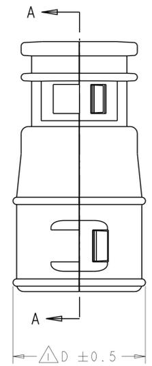
△ DIMENSION TO BE MEASURED WHEN THE COVER IS CLOSED.
