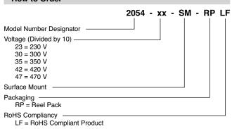
Model 2054-xx-SM-RPLF (Reel Pack) contains 900 pieces per reel, 2,700 pieces per box. The reel is 330 mm in diameter and 18 mm wide.
