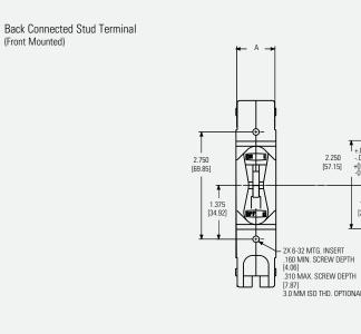
Note: Tolerance ± .015 [.38] unless noted. Dimensions in brackets [ ] are millimeters
