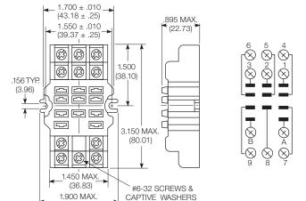
Screw terminal, DIN rail, snap-mount socket 27E893
