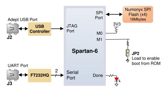
An on-board mode jumper (JP2) selects between JTAG/USB and ROM programming modes. If JP2 is loaded, the FPGA will automatically configure itself from the ROM. If JP2 is not loaded, the FPGA will remain idle after power-on until configured from the JTAG port.
