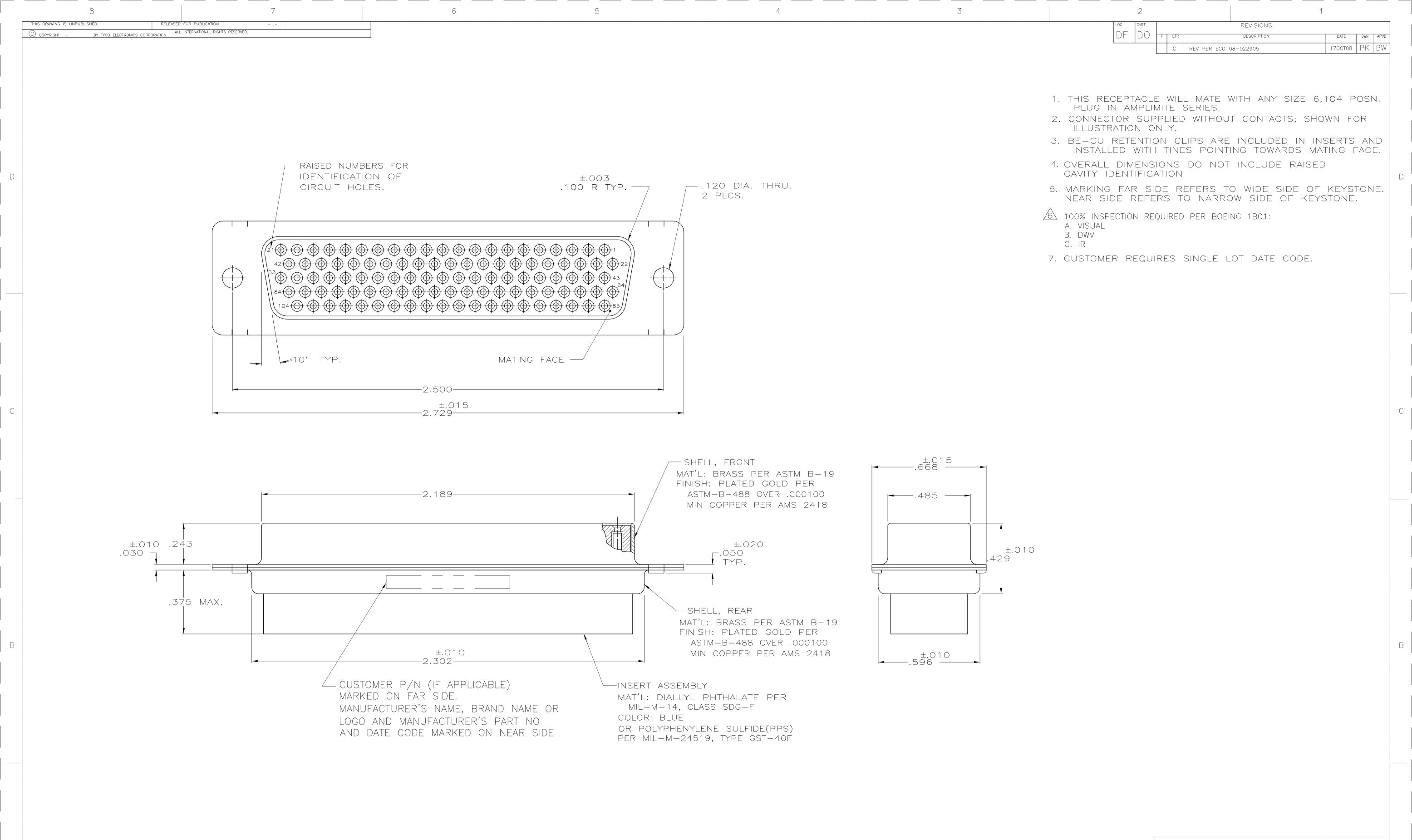
REMARKS CUSTOMER PART NUMBER PART NO. THIS DRAWING IS A CONTROLLED DOCUMENT. Tyco Electronics Corporation 4/26/84 Harrisburg, PA 17105-3608 TOLERANCES UNLESS OTHERWISE SPECIFIED: INCHES RECEPTACLE ASS'Y, AMPLIMITE 104 POSN, SIZE 6, SERIES 90 2 PLC ± -3 PLC ± .005 4 PLC ± -NON-MAGNETIC PPLICATION SPEC SIZE CAGE CODE DRAWING NO 41 00779 **C-**211648 SEE CALLOUT SEE CALLOUT SCALE NTS SHEET 1 OF 1 REV C JSTOMER DRAWING
