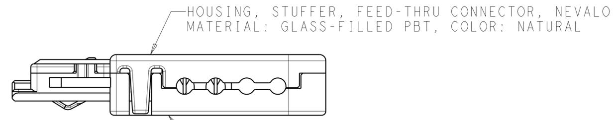
SUB-ASSEMBLY, BASE, FEED-THRU CONNECTOR, NEVALO
