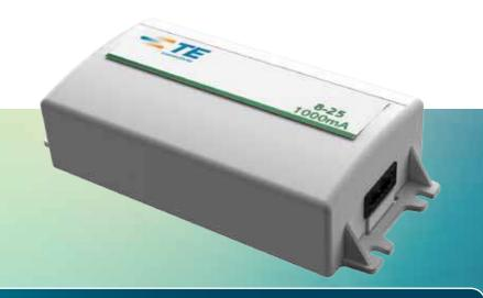
The NEVALO 25W triac dimmable LED driver is a high efficiency, power factor corrected supply with a unique color coded, keyed interconnect design that ensures optimal power is delivered to LEDs. The driver is designed with built-in voltage and thermal protection and is warranted for 5 years when used with the NEVALO SSL System.
