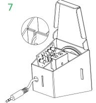
Slot the audio jack through the hole, insert electronics into the designated compartments & ensure wires are sat in the notches provided.
