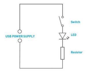
The circuit diagram for the USB lamp is shown above. It is a very simple circuit. The 5V that powers the circuit is supplied from the micro USB connector.
