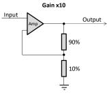
With an infinite gain the amplifier is no good to amplify audio, which is where the feedback comes in. By making one of the inputs a percentage of the output the gain can be fixed, which allows the output to be a copy of the input but bigger. Now when the two inputs are compared and the output is adjusted, instead of it going up or down until it reaches 0 volts or V+, it stops at the point when the two inputs match and the output is at the required voltage.
