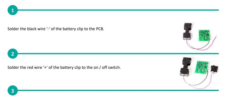
Using a piece of red wire, solder the remaining terminal on the on / off switch to the remaining power connection on the PCB.
