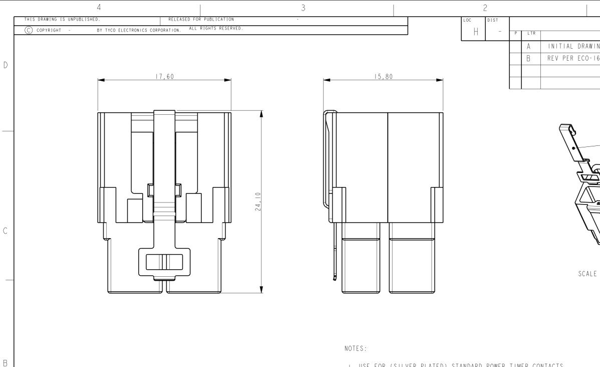
I USE FOR (SILVER PLATED) STANDARD POWER TIMER CONTACTS . FOR CONTACTS PARTNUMBERS SEE DWG. C-I355048 VERSION A ALLOWED MAX WIRE SIZE IOAWG.
