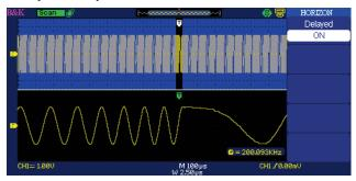
Use the oscilloscope's delayed sweep feature to zoom in a particular area of a signal in real time while viewing the entire captured waveform simultaneously.
