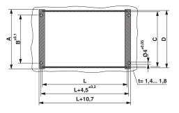
L = length of cover required; dimensions A=76 mm; B=58 mm; C=69 mm; D=73 mm
