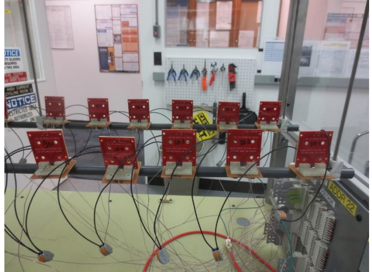
Figure 2 Temperature Rise Set Up
