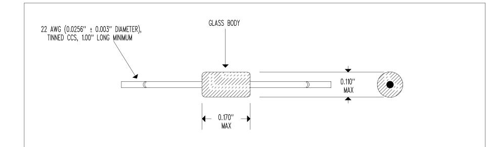
RESISTANCE @  $+25^{\circ}C = 2,252 \Omega \pm 10\%$ RESISTANCE TEMPERATURE CURVE = "J" BETA " $\beta$ " (0 TO  $+50^{\circ}C$ ) = 3,892'K NOMINAL TEMPERATURE COEFFICIENT @  $+25^{\circ}C = -4.4\%$ /°C NOMINAL DISSIPATION CONSTANT = 3 mW/°C NOMINAL (STILL AIR) THERMAL TIME CONSTANT = 8 SECONDS NOMINAL (STILL AIR) THERMAL TIME CONSTANT = 2 SECONDS NOMINAL (STIRRED OIL) MAXIMUM TEMPERATURE RATING =  $+300^{\circ}C$
