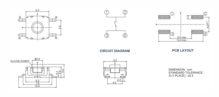
Figure 2 – 222JJA, Surface Mount J-Bend Terminal, Actuator Height 3.5mm
