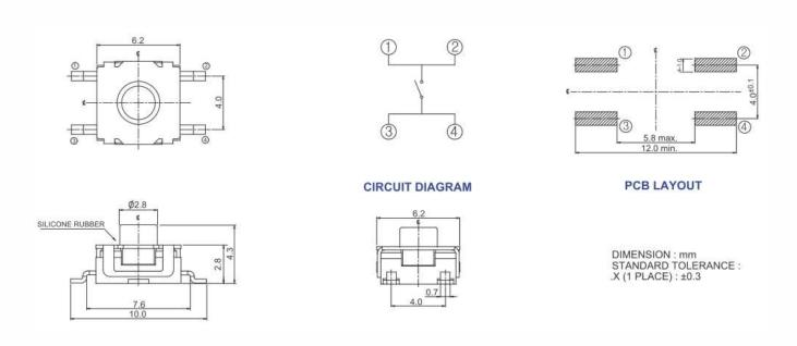
Figure 2 – 222LJA, Surface Mount J Bend, Actuator Height 4.3mm
