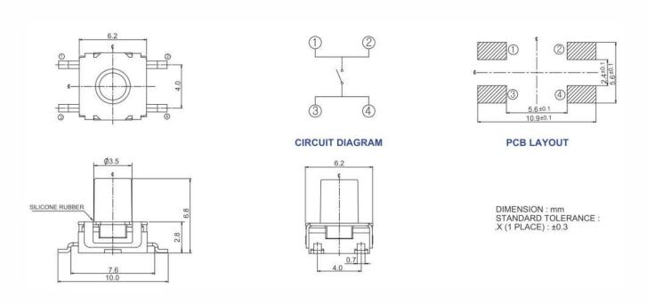
Figure 2 – 222MJA, Surface Mount J Bend, Actuator Height 6.8mm
