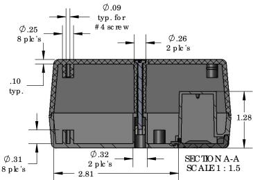
DESCRIPTION 2-2R BOTTOM 319 Prototype Grid Circuit board BATTERY COVER 419 Prototype Clad Circuit board 6018 4-40 SCREW (2) 6102 THREADED INSERTS (2)
