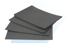
Q-ZORB PN 2238, RFSW-S-040-FR is a flexible elastomeric magnetic absorbing material. The material is designed to perform well for surface current attenuation. It can be used to lower the Q of cavities and reduce EMI. It is easily bonded using contact adhesives or it can be supplied with a pressure sensitive acrylic adhesive (PSA).
