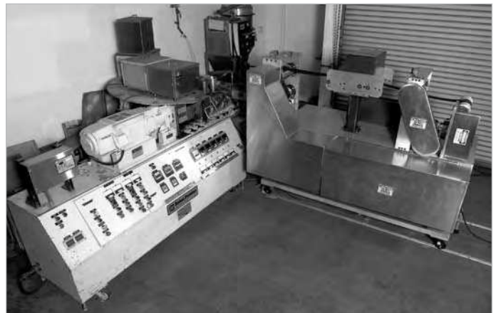
Thermoplastic extruder for microwave absorbing thermoplastic products.
