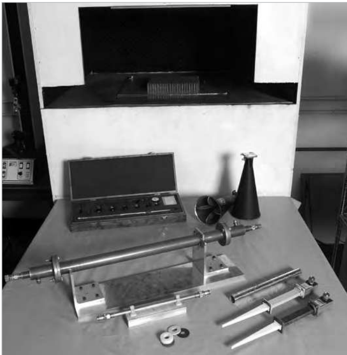
▲ Transmission tunnel and microwave test equipment for material property measurement.
