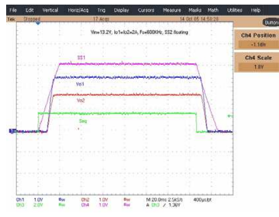
Fig. 13: Ratiometric Power up /down
