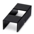
Secondary terminal cover to increase air and creepage distances when installed horizontally, length of 75 mm for PACT MCR-V2-3015-60-... and PACT MCR-V2-5012-85-...
