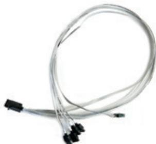
The Adaptec I-HDmSAS-4SATA-SB-.8M is an internal mini SAS HD x4 (SFF-8643) to (4) x1 Serial ATA (adapter based) fan-out cable with sideband signals. It measures 0.8 meters and is used for connecting a Series 7/7Q/7H adapter to SATA disks, or a SAS/SATA backplane.
