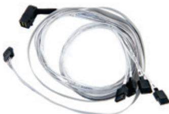
The Adaptec I-rA-HDmSAS-4SATA-SB-.8M is an internal "right angle" mini SAS HD x4 (SFF-8643) to (4) x1 Serial ATA (adapter based) fan-out cable with sideband signals. It measures 0.8 meters and is used for connecting a Series 7/7Q/7H/7He adapter to SATA disks, or a SAS/SATA backplane.
