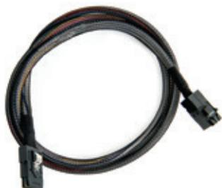
The Adaptec I-HDmSAS-mSAS-1M and .5M are internal mini SAS HD x4 (SFF-8643) to mini SAS (SFF-8087) x4 cable. They measure 1 or 0.5 meters and is used for connecting a Series 7/7Q/7H adapter to a SAS/SATA backplane.
