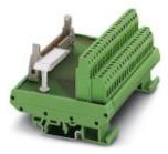
VARIOFACE module, with screw connection and flat-ribbon cable connector, for mounting on NS 32 or NS 35/7.5, with pin strip and short and long locking latches for socket strips. 60-pos.
