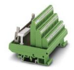
VARIOFACE module, with screw connection and flat-ribbon cable connector, for mounting on NS 32 or NS 35/7.5, with pin strip and short and long locking latches for socket strips, 16-pos.
