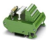
VARIOFACE module, with spring-cage connection and one D-SUB miniature pin strip, integrated PE contact for connecting the PCB and DIN rail, 15-pos.
