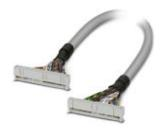
Round cable set; connection 1: IDC/FLK socket strip (1x 34-position); connection 2: IDC/FLK socket strip (1x 34-position); cable length: 3 m
