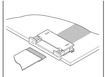
This extremely small 0.5mm pitch connector with a height of only 2.0mm above the PCB surface allows interconnection in extremely small spaces and is an example of JST's leading edge technology.
