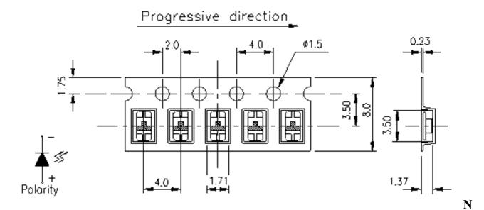
ote: The tolerances unless mentioned is  $\pm 0.1$ mm ,Unit = mm
