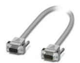
Assembled shielded round cable; connection 1: D-SUB socket strip (1x 9-position); connection 2: D-SUB pin strip (1x 9-position); cable length: 6 m
