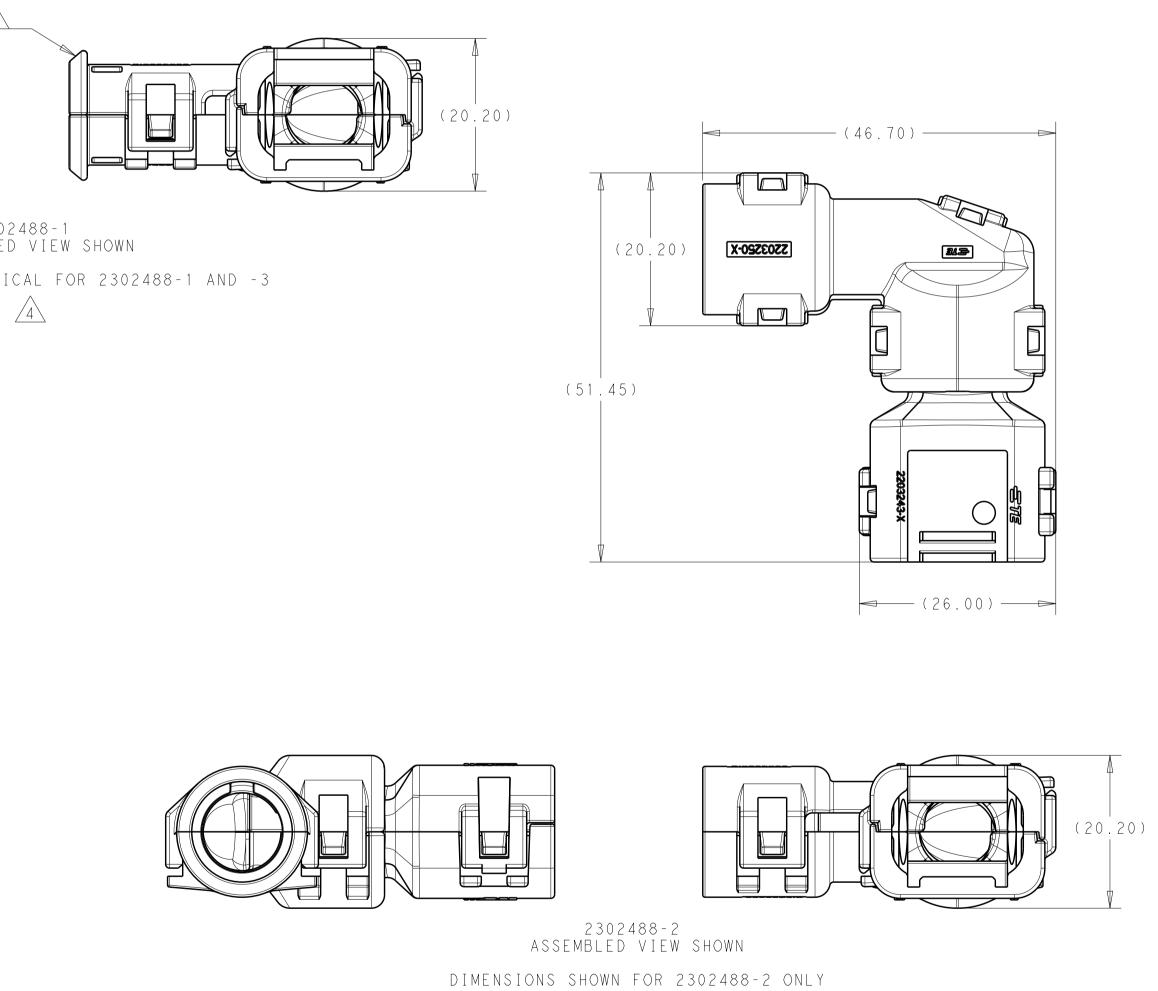
2302488-1 Assembled view shown DIMENSIONS SHOWN TYPICAL FOR 2302488-1 AND -3
