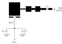
= Microstrip on 0.020" Duroid, Er=2.55 C1, C2 = 68pF ATC "A" C3 = 10MFD @ 35V
