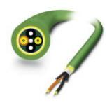
PROFINET HCS GI fiber cables, duplex 200/230 µm, increased bandwidth for Ethernet applications in particular. Robust PUR outer sheath. Heavy version suitable for drag chains and indoor installation, sold by the meter without plugs
