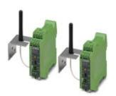
Bluetooth PROFIBUS SET, pre-configured: PROFIBUS point-to-point, PROFIBUS baud rate: 187.5 kbps, integrated path diagnostics: bar graph + two digital outputs, cross-wiring of 24 V DC and RS-485 2-wire, contents: 2 x Bluetooth converter + 2 x antenna
