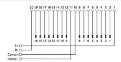
FLKM 16-PA-S300/MINI-MCR connection scheme
