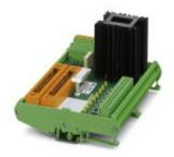
8-channel digital output module with spring-cage connection. The power supply unit and the 50-pos. strip are designed redundantly. Suitable for Yokogawa card SDV 531 and SDV 531L.
