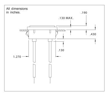
Mounting: Will snap-fit into Ø.032/.100 thick panels. Use speednut for other panel thicknesses.
