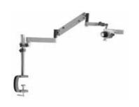
The Articulating Arm with Vertical Extension is 34" in length, has a 12" vertical range of motion and a maximum clearance of 16" above the benchtop surface. Includes a heavy-duty clamp that opens 4" wide in order to accommodate workstations or bench edges. For use with all Luxo System 273 and 373 microscopes.
