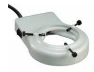
Fluorescent Ring Light provides full illumination with a powerful 17-watt, 5600°K lamp. A durable powder-coated metal housing protects the fluorescent lamp which has a rated lamp-life of 4,500 hours and produces 2,000 footcandles at 4.5" working distance.. Plug-in ballast with polarized plug is included.
