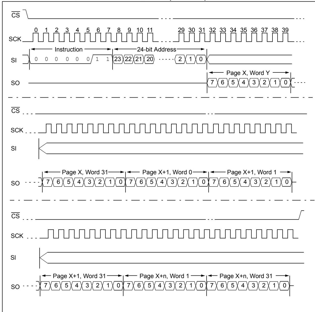
**FIGURE 2-6: SEQUENTIAL WRITE SEQUENCE (SPI MODE)**
