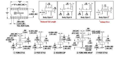
ALL DIMENSIONS: INCHES [MILLIMETERS] ALL TOLERANCES: ±0.005 [0.13] UNLESS OTHERWISE SPECIFIED CONSULT FACTORY FOR OTHER SIZES AND CONFIGURATIONS CUSTOMIZATION: ARIES SPECIALIZES IN CUSTOM DESIGN AND PRODUCTION. SPECIAL MATERIALS, PLATINGS, SIZES, AND CONFIGURATIONS CAN BE FURNISHED, DEPENDING ON QUANTITY.
